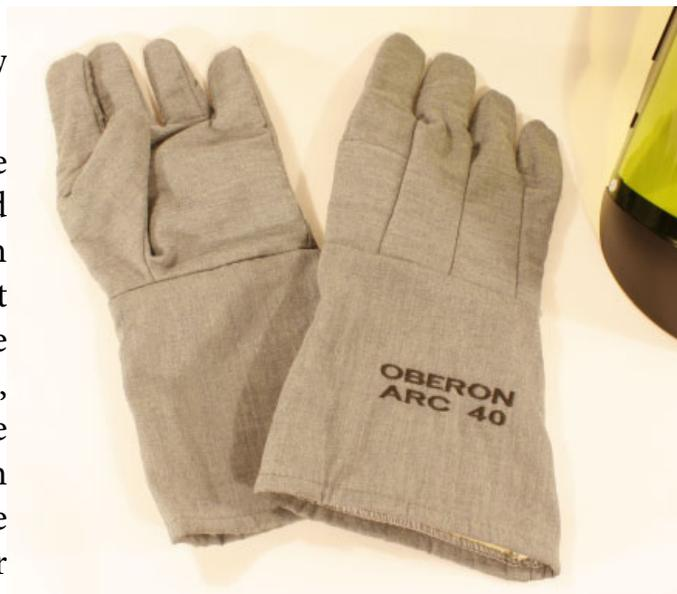
Arc Flash Gloves are NOT manufactured of rubber. As such, they do not provide shock protection against voltage. They should not be used within the Prohibited Approach Boundary as defined by NFPA 70E where there is the risk of contact with voltage due to proximity to the energized circuit. Within this space, only Rubber Electrically Insulating Gloves should be used to protect the worker from accidental electric shock.
