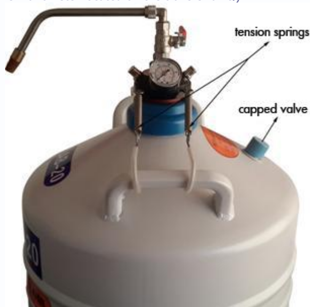
R.09[[ Transfer unit tension springs and tank capped valve ]]
