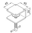
MOUNTING CLAMP ML311 MOUNTING ANGLE PLATE ML137
