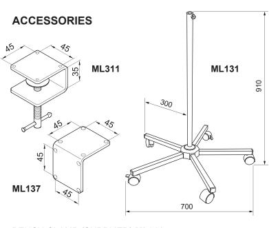
BENCH CLAMP (SUPPLIED) ML311 WALL BRACKET ML137 MOBILE STAND ML131
